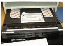
This device allows users to read in braille what is displayed on a computer screen or print such information in braille.
